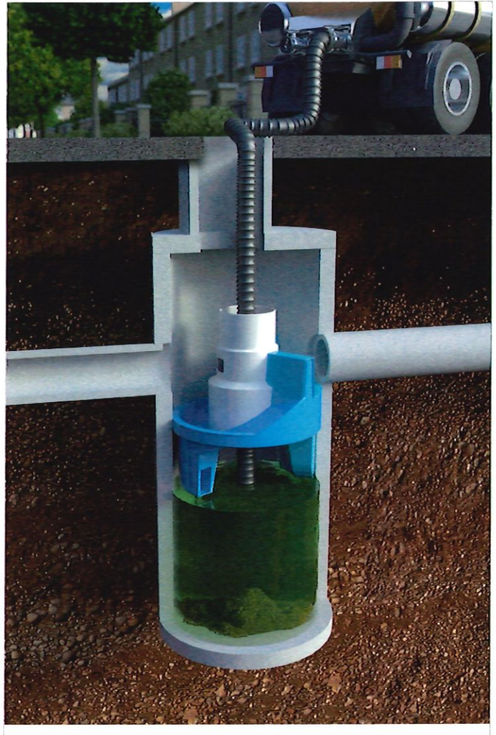
Fig.4 Floatables are removed with a vector hose
