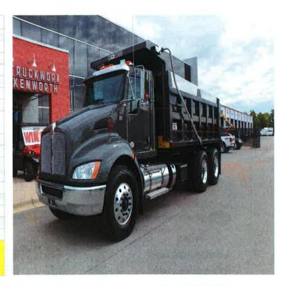
Only offered on Kenworth Model Trucks: Bulkhead doors, fully huck-bolted cab(s), cowl mounted mirrors, rear/driver corner windows, and peeper windows. The above specifications are offered for safety and durability purposes.
