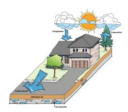
In post-development conditions only 10-50% of rainwater infiltrates into groundwater.
