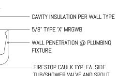
TUB/SHOWER VALVE AND SPOUT PENETRATIONS SHALL BE PROTECTED PER UL FIRESTOP.
