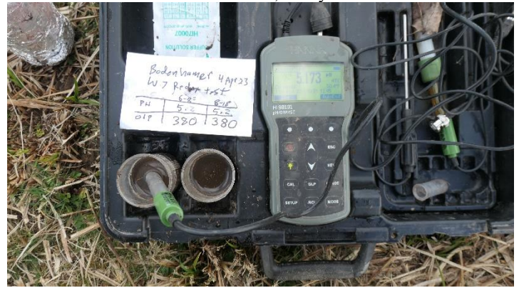
Photo 80. Redox Test at Piezometer W7, Study Area C
