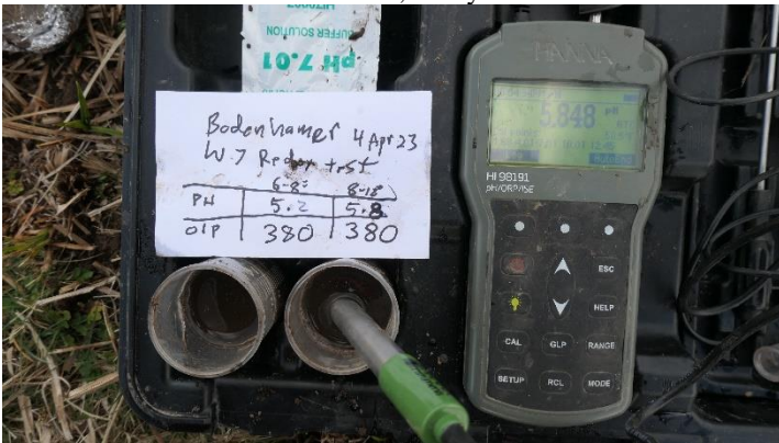
Photo 81. Redox Test at Well W7, Study Area C
