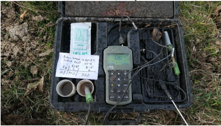
Photo 79. Redox Test at Well W4, Study Area B
