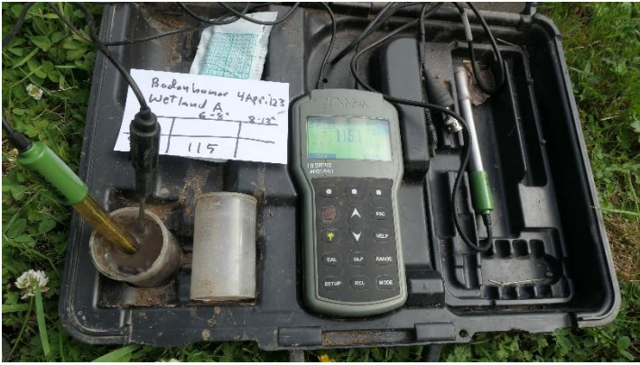
Photo 85. Redox Test Positive at TP-A1 in Wetland A
