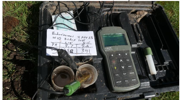
Photo 82. Redox Test at Well W10, Study Area D
