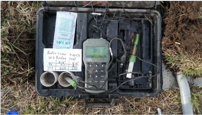
Photo 77. Redox Test at Well W2, Study Area A
