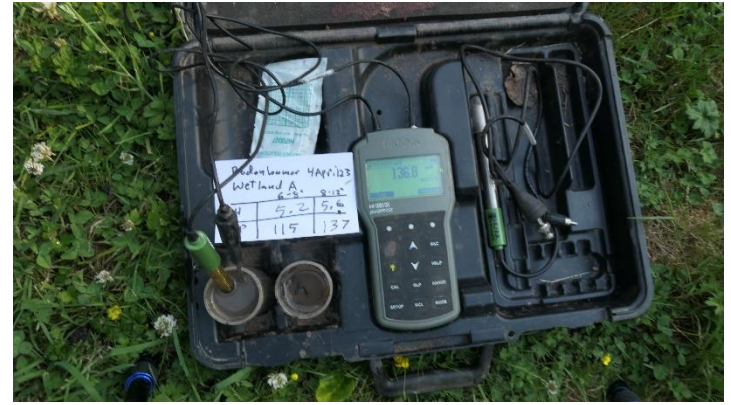
Photo 86. Redox Test Positive at TP-A1 in Wetland A
