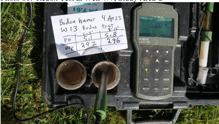
Photo 83. Redox Test at Well W13, Study Area E
