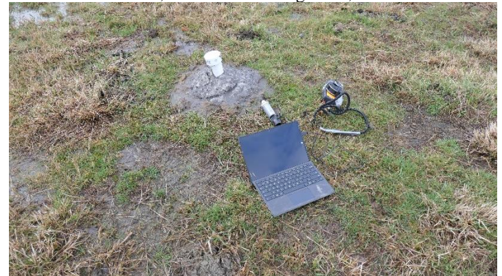
Photo 54. Collecting well data in the field from dataloggers
