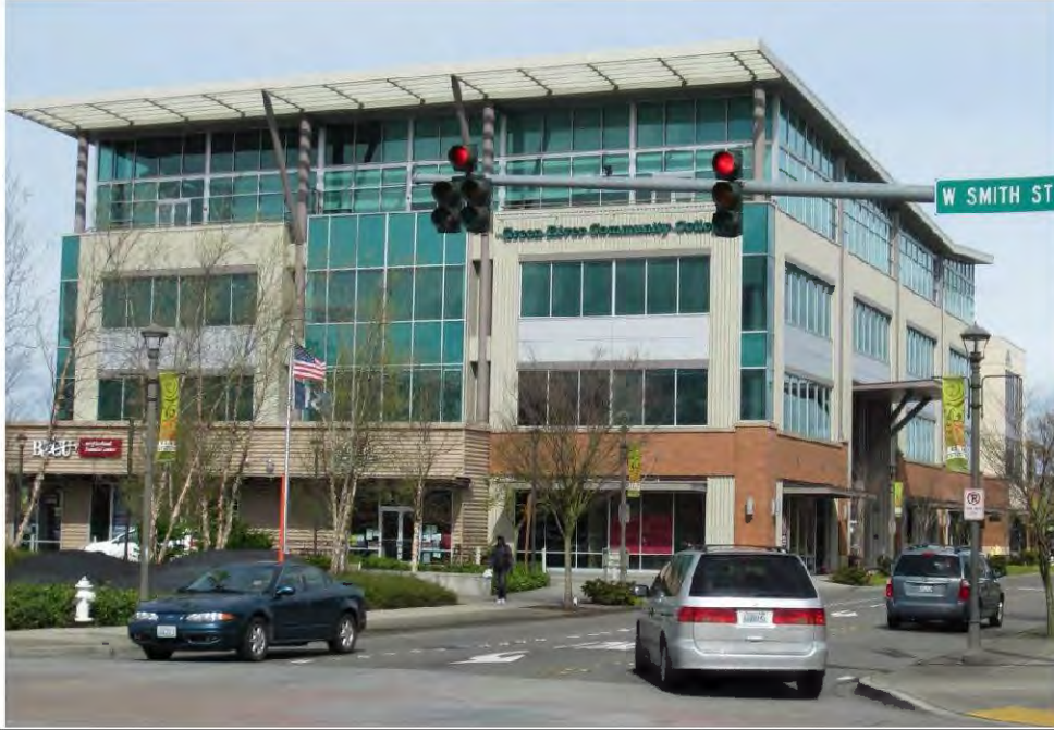
4.B.6.2-2. Green River Community College incorporates passive surveillance, territorial definition, active ground floors, and good visibility and lighting to provide a secure open space in front of their building.
