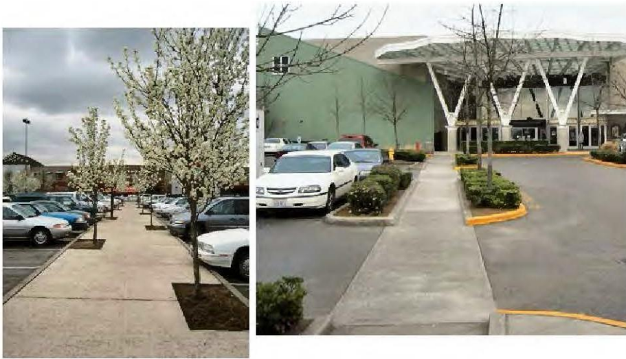
Figure 2.D.1.1-1. Parking area pathway examples. Note that clear pathway width must account for vehicle overhang.
