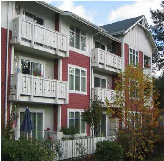
Figure 2.E.6.1-2. The multifamily building provides a number of details that enhance the pedestrian environment, including decorative railing, different siding treatments, window trim, balconies, eave detailing, lights, and opportunities for individual landscaping.
