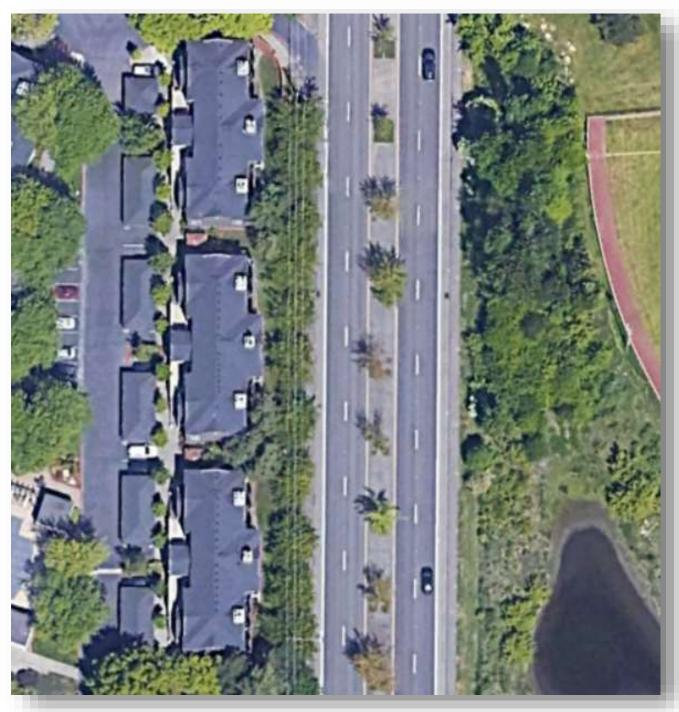
Placing the parking between roadway and receiver will reduce noise!
