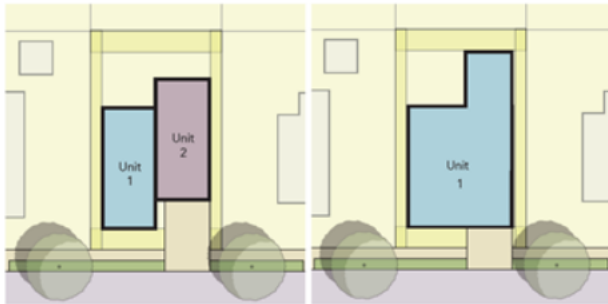
Figure 1: Duplex and Detached Single Family structures occupying similar footprints, setbacks, and massing.
