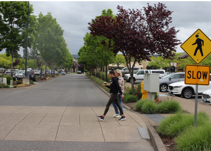
DO Define safe crossings for pedestrians with changes in grade, materials, speed bumps, signage, and other means to slow down vehicular traffic.
