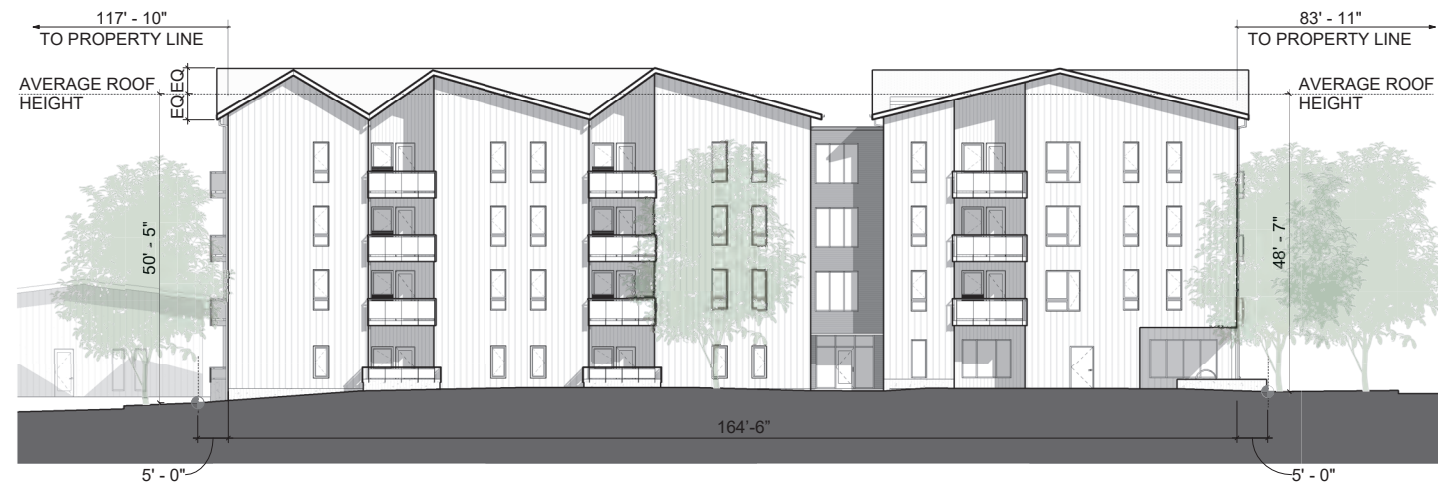
SOUTH ELEVATION | BUILDING A NOT TO SCALE
