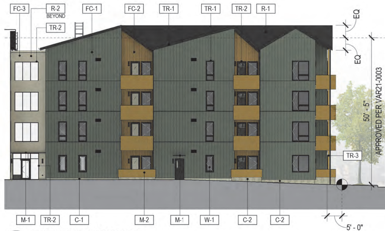
2 BUILDING A - NORTH SIDE SCALE: 1" = 20'-0"
