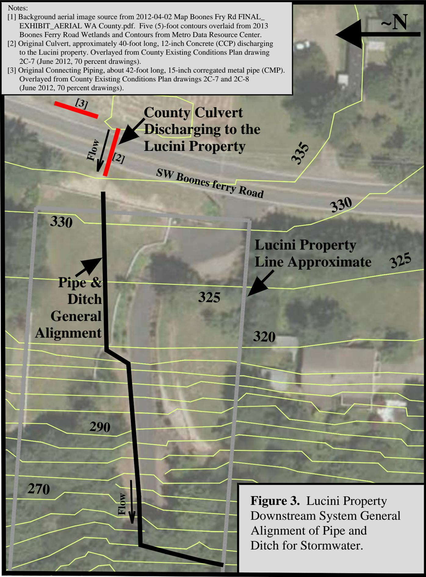
**Figure 3.** Lucini Property Downstream System General Alignment of Pipe and Ditch for Stormwater.
