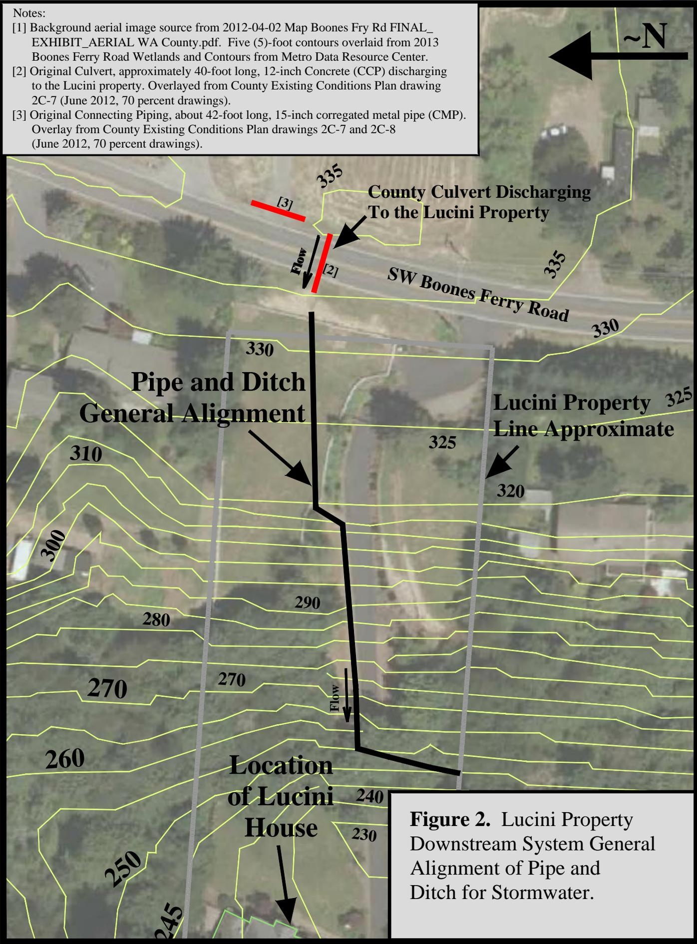
**Figure 2.** Lucini Property Downstream System General Alignment of Pipe and Ditch for Stormwater.
