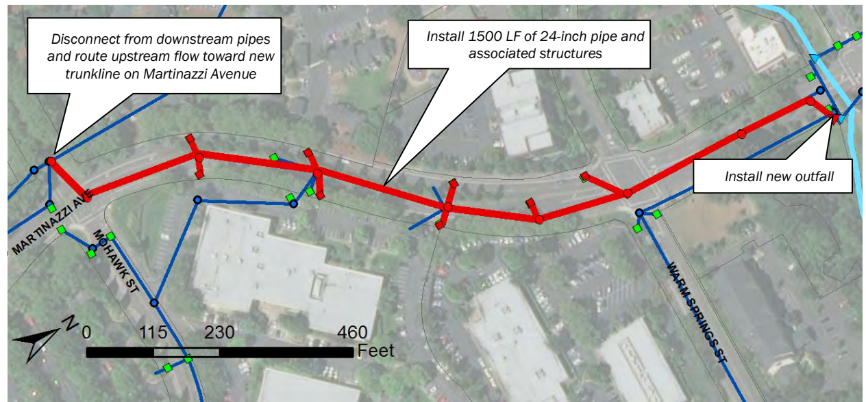
Figure 1. Construction details of Phase 1
