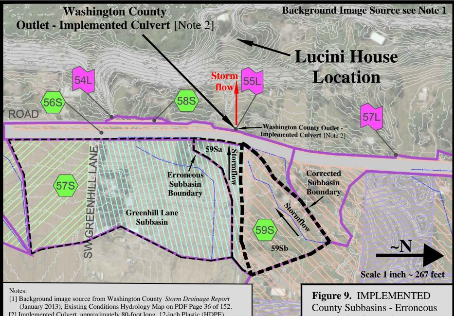
[2] Implemented Culvert, approximately 80-foot long, 12-inch Plastic (HDPE) discharging to the Lucini property. Overlayed from As-built construction plan drawings 232-233 of 385.
