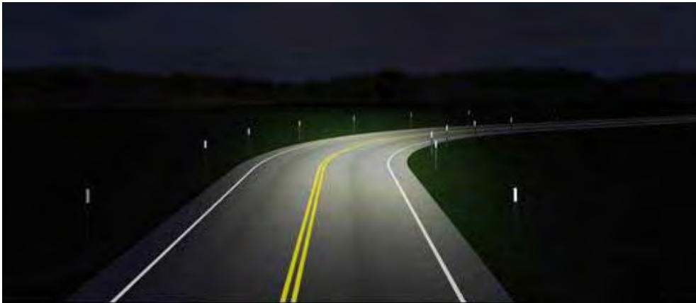
Figure 37: Example Delineators on Curved Roadway
