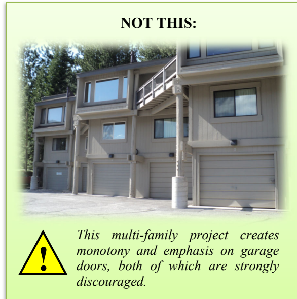
FIGURE 2-36 DISCOURAGED MULTI-FAMILY BUILDING DESIGN
