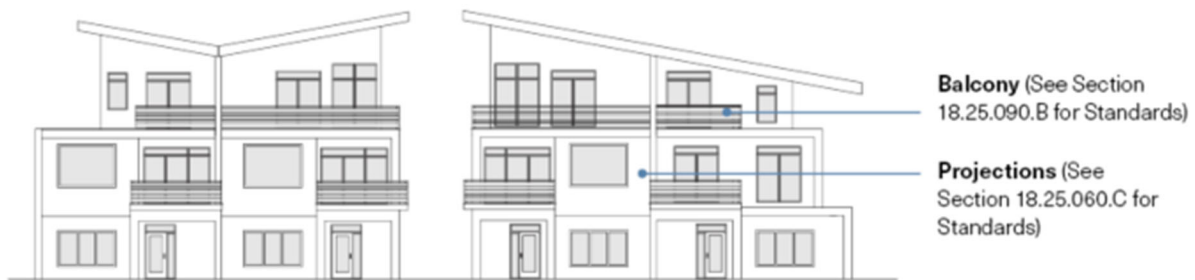
FIGURE 2-X INDIVIDUAL BUILDING BALCONIES AND PROJECTIONS
