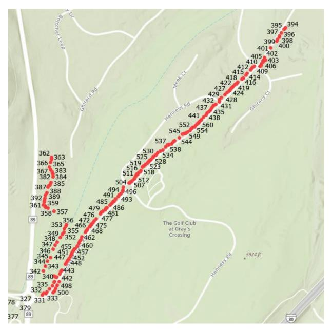
Map shows individual cracks along the Prosser Dam Road Trail and the SR 89 Trail. The Cracks proposed to be repair without an overlay.
