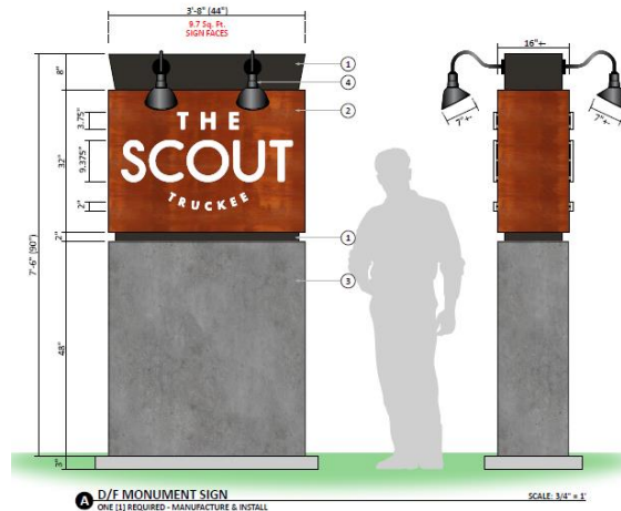
Figure 12: Current building permit ground-mounted sign design (located at the east entrance along Edwin Way)
