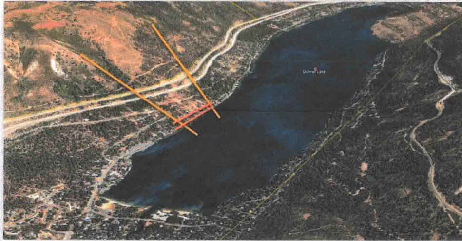
The focus of this report is a hillside and drainage that is unique in the Lake basin due to the extreme lack of vegetation, its length and steepness, its erodability, and the concentration of freeway drainage all funneling stormwater (sediment and pollutants) runoff down to and sometimes into the homes of the residents of Reed Avenue West and Donner Pass Road, shown in orange, and then into Donner Lake.
