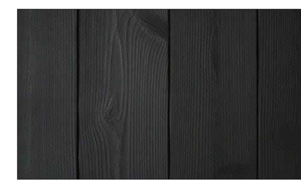
D VERTICAL WOOD SIDING ROUGH SAWN, STK COLOR: DARK CHARCOAL WUJ COMPLIANT
