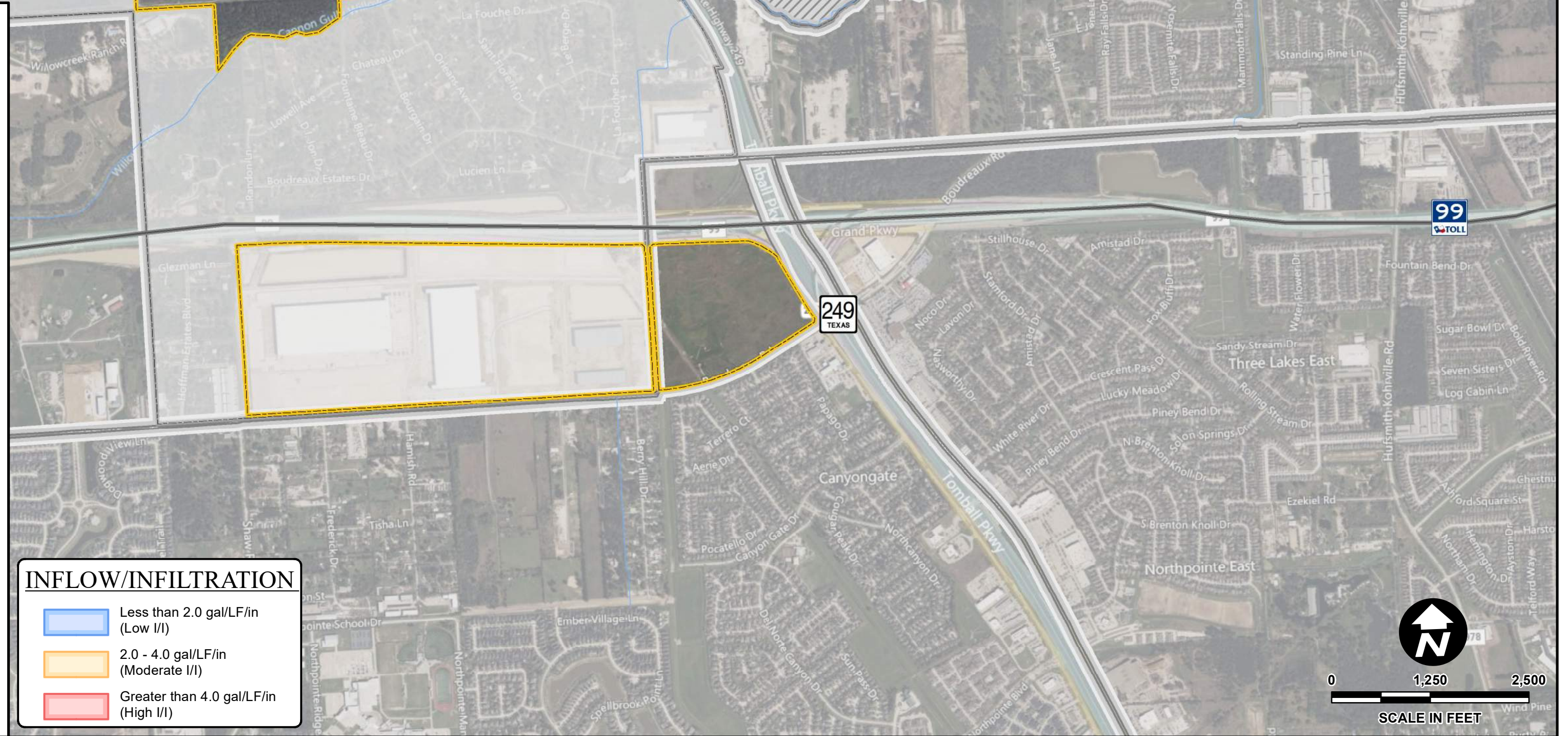
FIGURE 8-5 CITY OF TOMBALL 2023 WATER AND WASTEWATER MASTER PLAN UPDATE NORMALIZED I/I BY FLOW METER BASIN (GAL/LF/IN) LEGEND Rain Gauge Grand Parkway 99 Flow Meter Stream Lift Station Unmonitored Basin Wastewater Treatment Plant ETJ Manhole Houston ETJ Boundary 8\" and smaller Wastewater Line City Limit 10\" and larger Wastewater Line County Line 8\" and smaller Force Main 10\" and larger Force Main THE CITY OF TOMBALL TEXAS FOUNDED 1907
