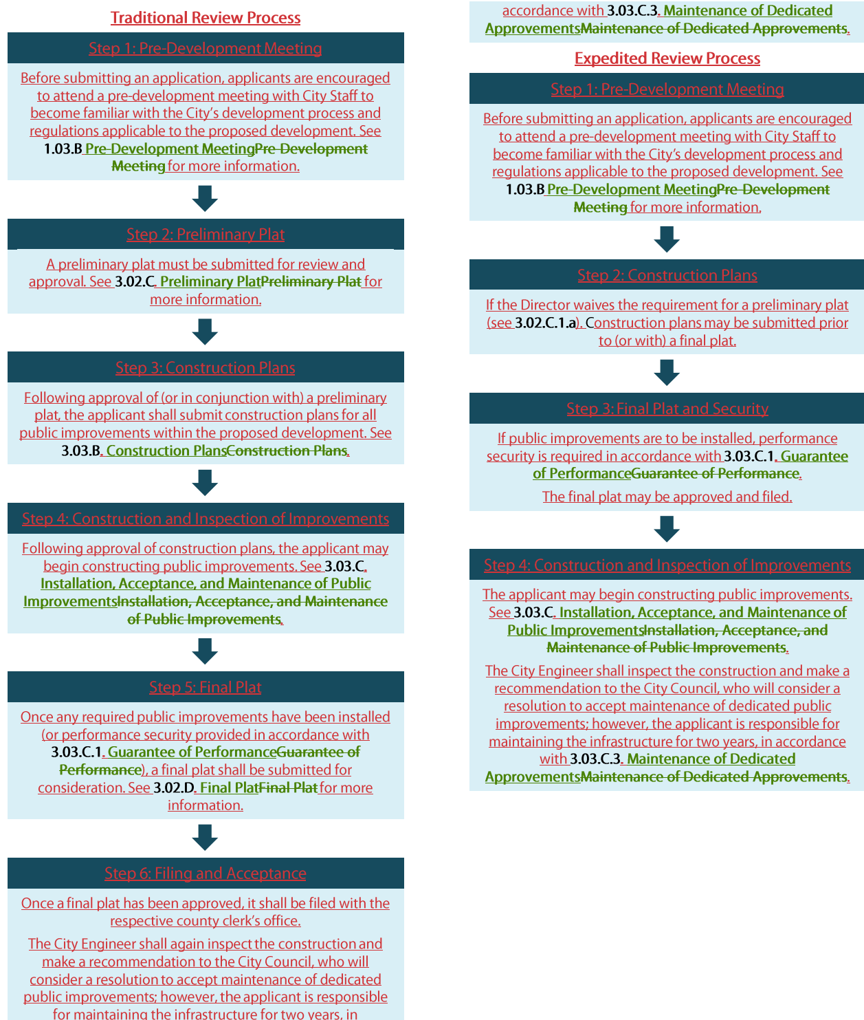
Figure 3.02-1. Platting Process Alternatives Overview
