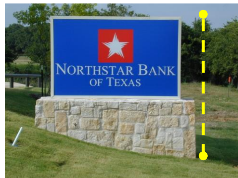
Figure 4.01-3. Sign Height Measurement
