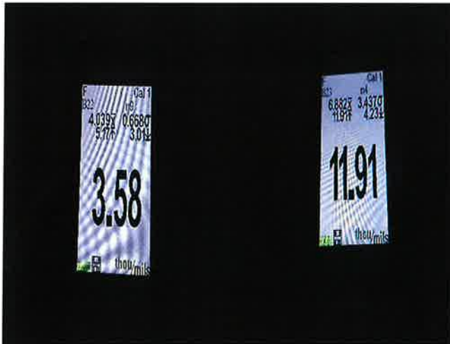
PRIMER DFT LOW AND HIGH READINGS
