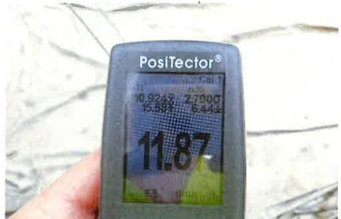
DFT READINGS, LOW/HIGH/AVG
