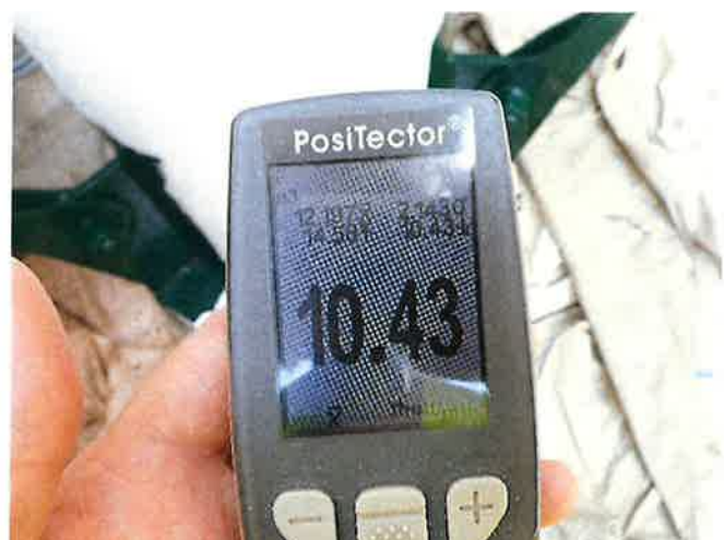
INTERMEDIATE COATING DFT READING
