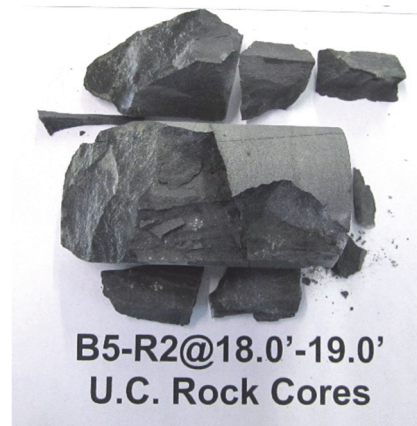
Photo 3: Test sample after testing
