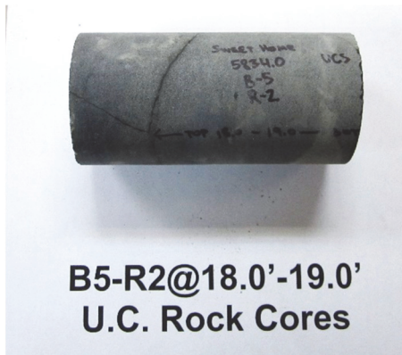
Photo 2: Test sample before testing
