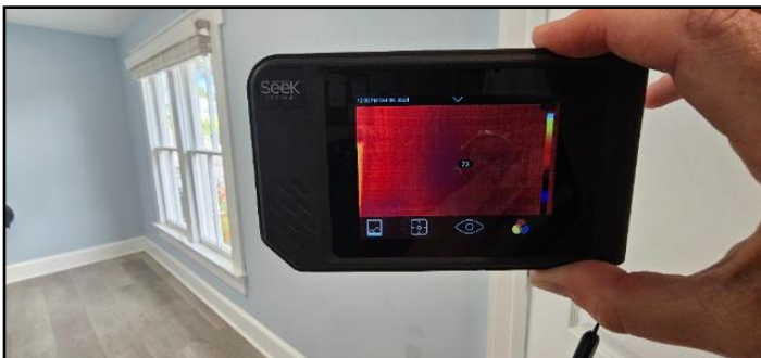
31. Moistuer in wall beside window
