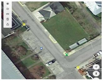
X = Remove and replace existing with Type 2 parallel curb ramp.
