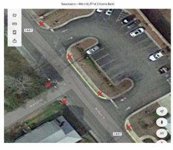
X = Remove and replace existing with Type 1 directional curb ramp.
