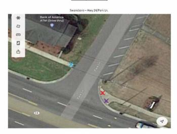
X = Remove and replace existing with Type 1 directional curb ramp.
