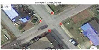
X = Remove and replace existing with Type 1 directional curb ramp.
