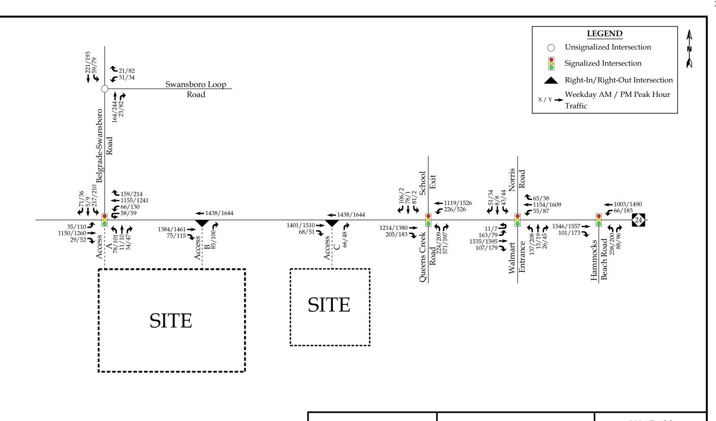
Note: Based on NCDOT Congestion Management guidelines, a volume of 4 vehicles per hour (vph) was analyzed for any movement with less than 4 vph.
