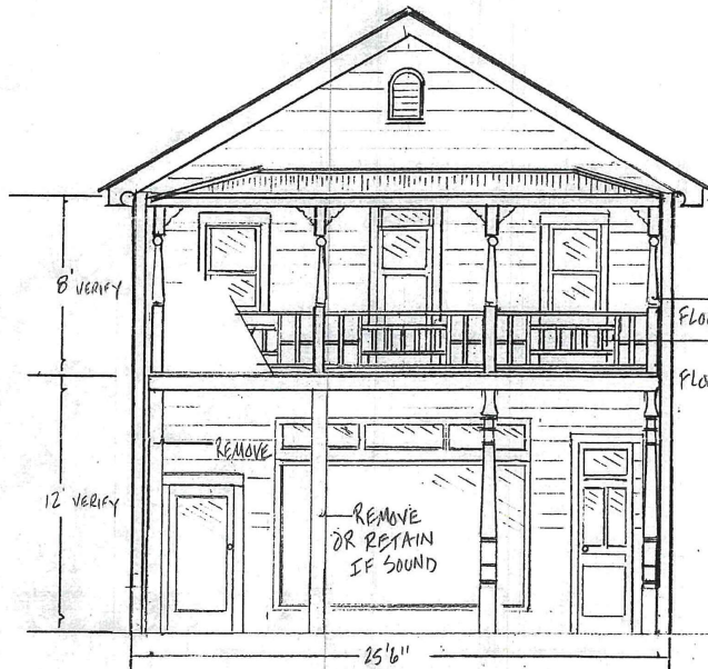
EXISTING FRONT ELEVATION 1/4"=1'
