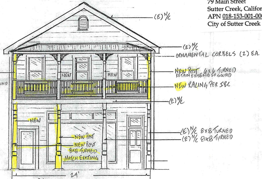
PROPOSED FRONT ELEVATION REPAIR 1/4"=1'
