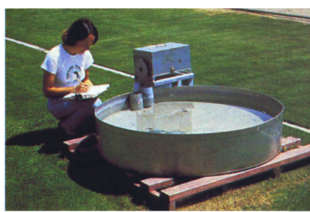
Class A Weather Bureau evaporation pan measured evapotranspiration from experimental turfgrass plots at the UC South Coast Field Station at Irvine.
