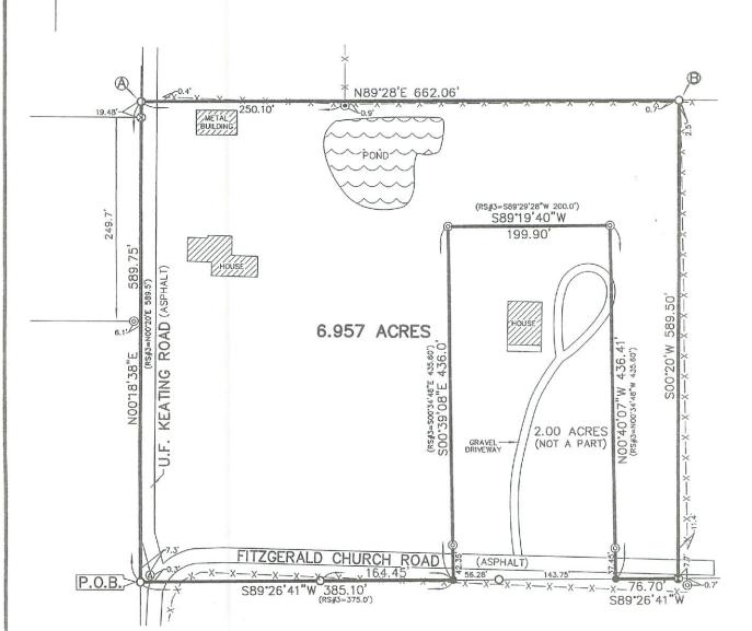
P.O.B. is reported to be East 1320.0' N00'20'E 1320.0' from the Section Corner common to Sections 28, 29, 32, & 33, T5S, R11E.
