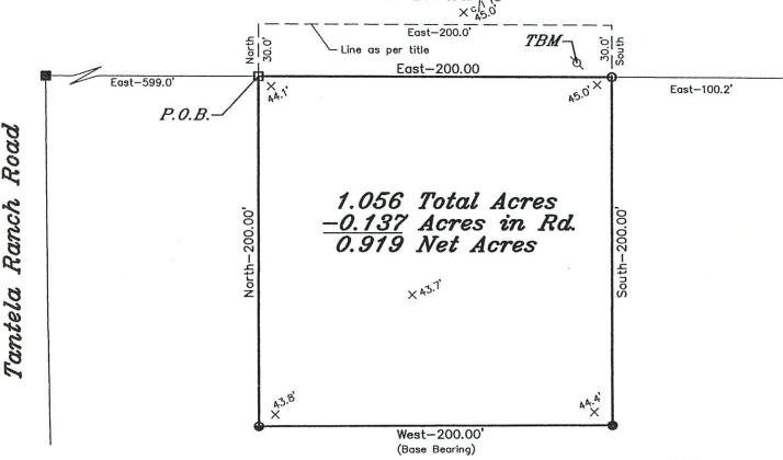
TBM: Nail set in Powerpole Elev. 47.1' Tag #2722 TBM is for reference only and does not represent the actual elevation to build to (Refers to NAVD 88 Geoid 18)
