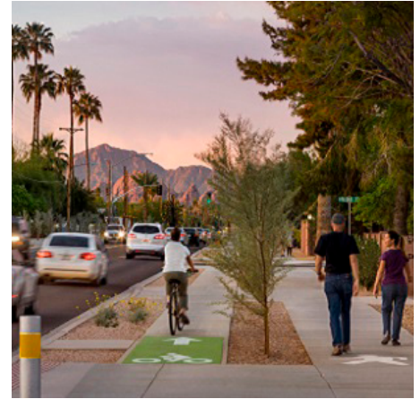
A shared use path buffered from travel lanes.
