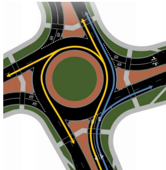
Illustrative roundabout showing traffic flow lines
