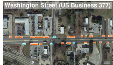
Excessive driveway access on busy arterial.
