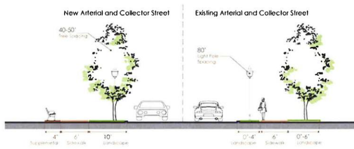
Streetscape Figure—Arterial and Collector Streets
