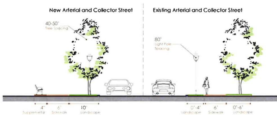
Streetscape Figure—Arterial and Collector Streets
