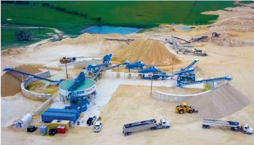
Exemplar: soil washing and screening plant
