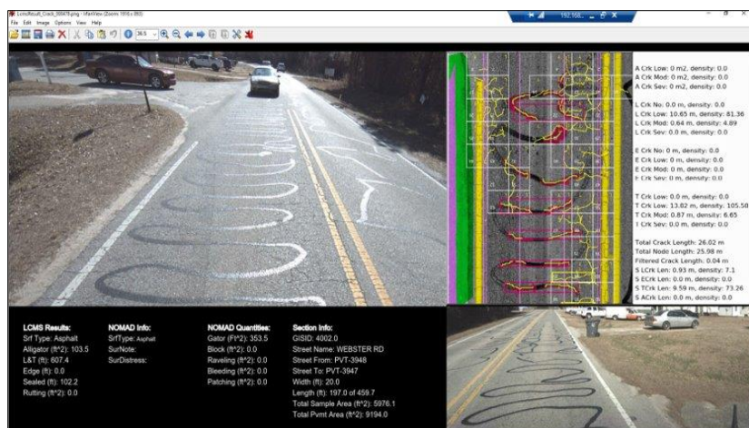
New QA Tool! IMS QC/QA interface for manually reviewing automated distress detection and classification results.
