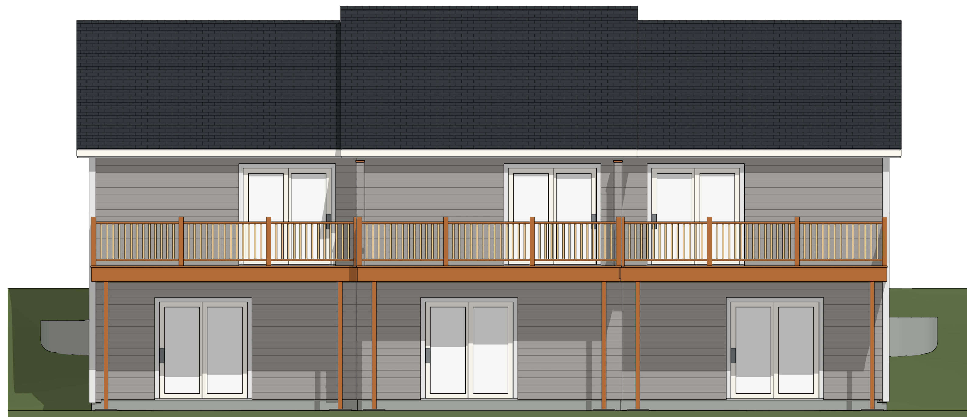
REAR ELEVATION SCALE: 1/4" = 1'-0"
