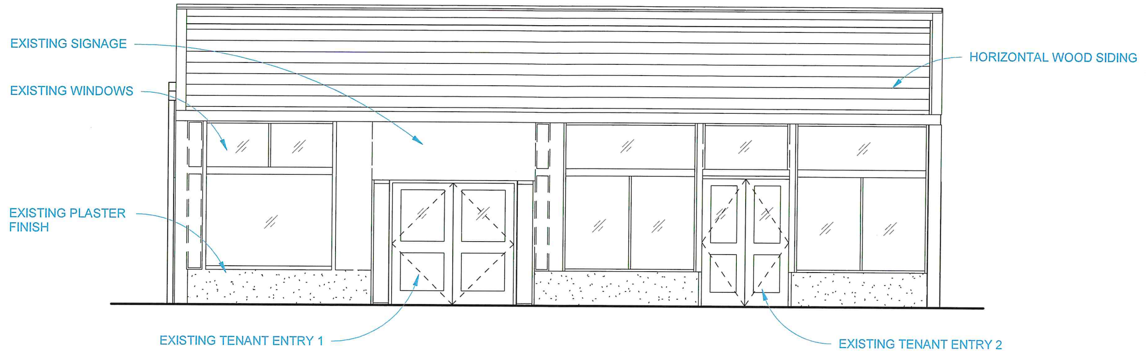
3 EAST ELEVATION EXISTING 3/16" = 1'-0"
