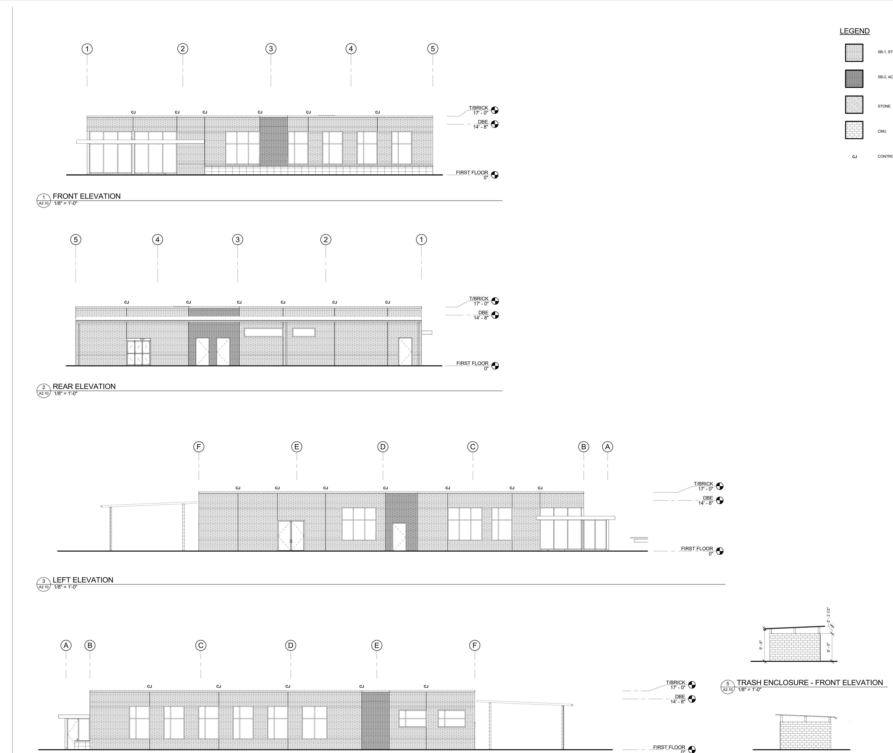
4 RIGHT ELEVATION A2.10 1/8" = 1'-0" SB-1, STRUCTURAL ATLAS BRICK 4X8X16
