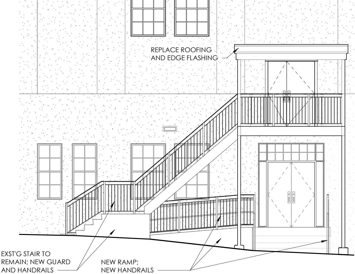
2 PROPOSED SOUTH STAIR SECTION 3/16" = 1'-0"
