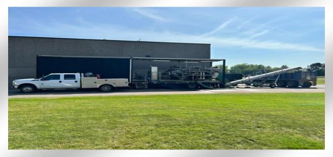
Fergus power pump processed about 900,000 gallons of liquid to produce about 300 tons of dry solids. The solids are pressed for a couple reasons, but the biggest reason is transportation. If a tanker transported the liquid for land application, it would take about 140 truckloads. By pressing the liquid to a solid, it only takes about 20 dump truck loads and costs a lot less.
