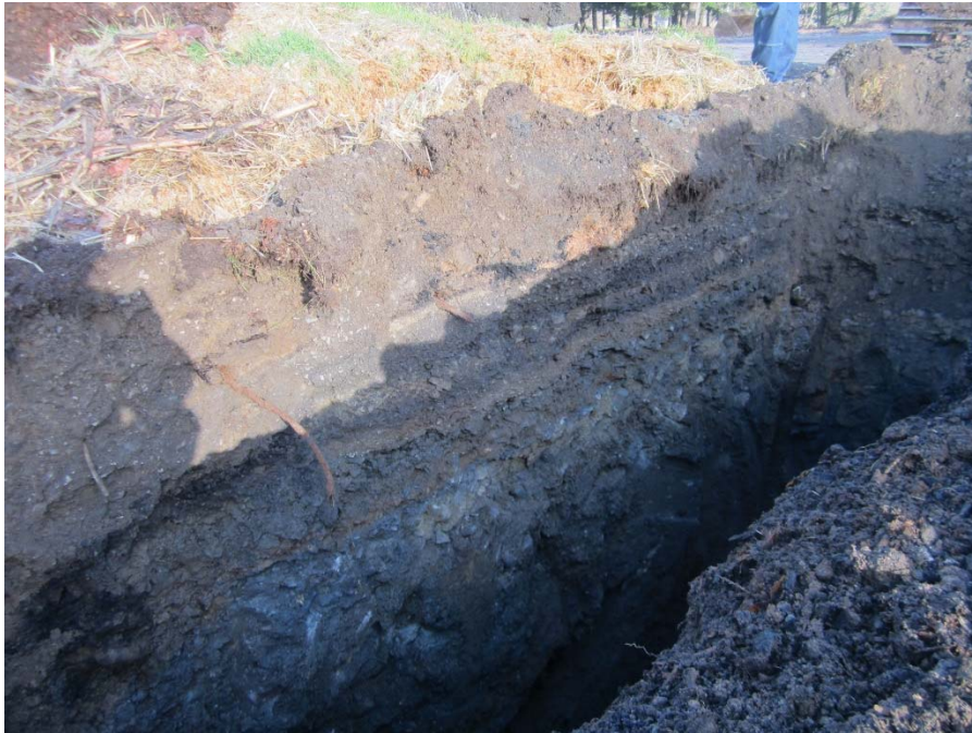
Photograph 4: Western sidewall of TP4, showing varied soil lenses in the upper 3 feet. Photograph taken facing northwest.
