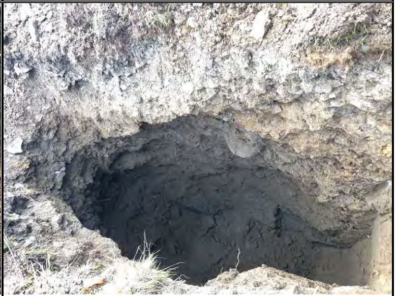
Exposed subsurface soil profile within test-pit TP-3
