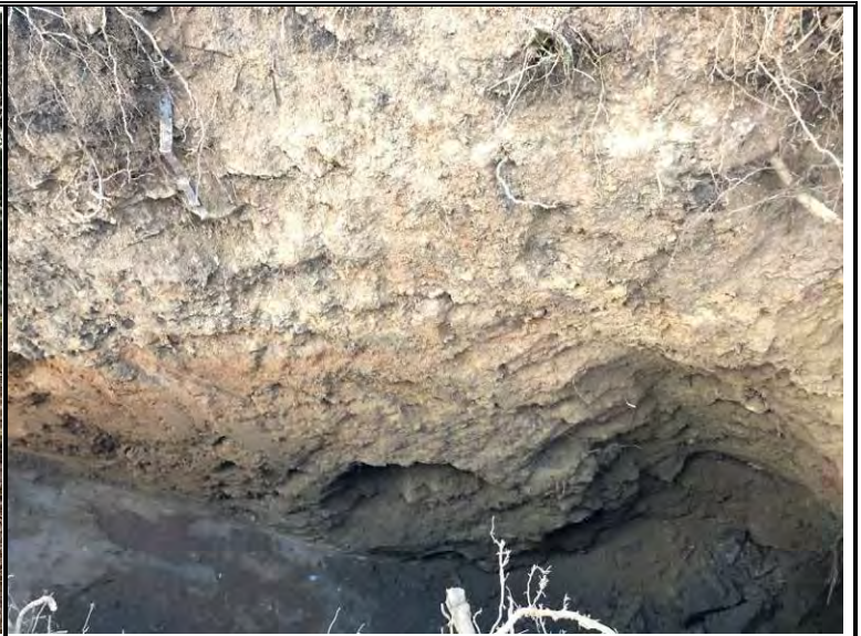
Exposed subsurface soil profile within test-pit TP-11
