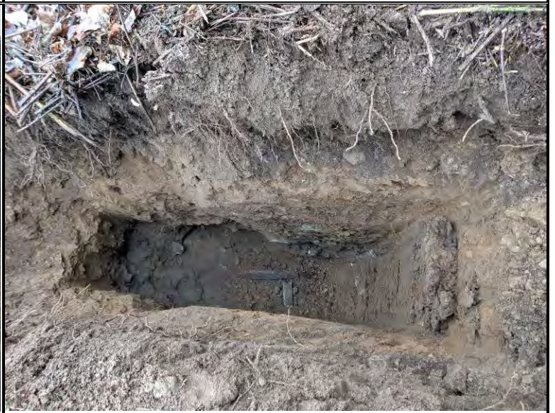
Exposed subsurface soil profile within test-pit TP-2
