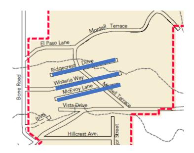
**#26 School Street Grind and Inlay**-Repair stormwater, replace waterlines, grind and inlay.
