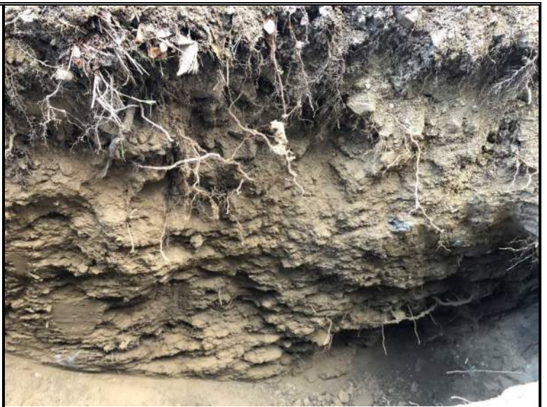
Exposed subsurface soil profile within test-pit TP-4
