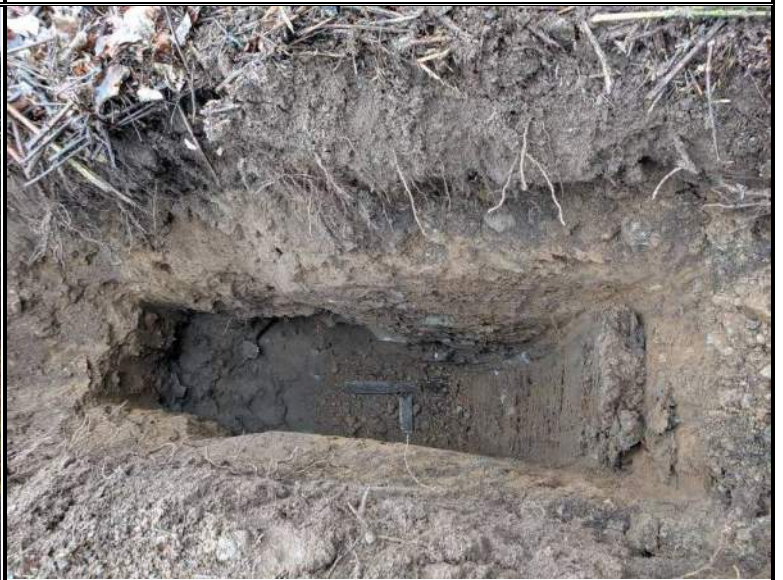
Exposed subsurface soil profile within test-pit TP-2
