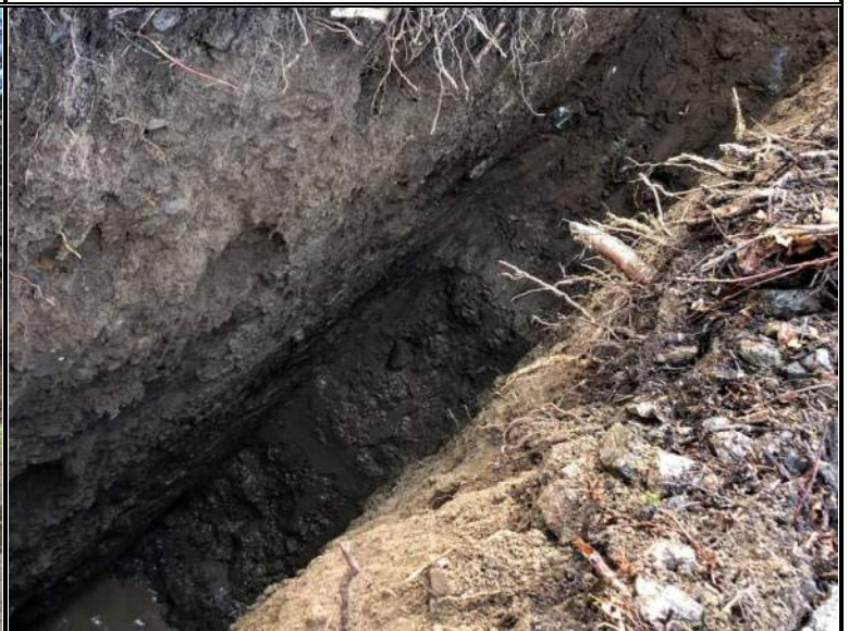
Exposed subsurface soil profile within test-pit TP-8
