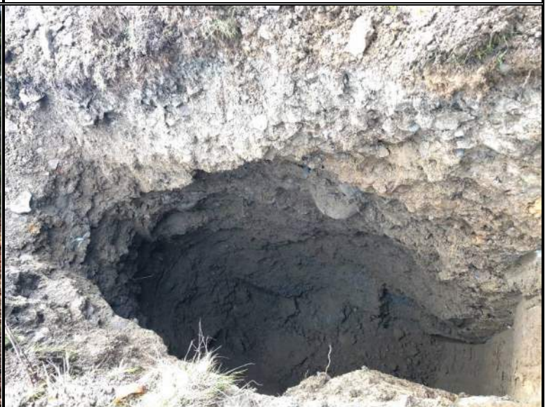
Exposed subsurface soil profile within test-pit TP-3
