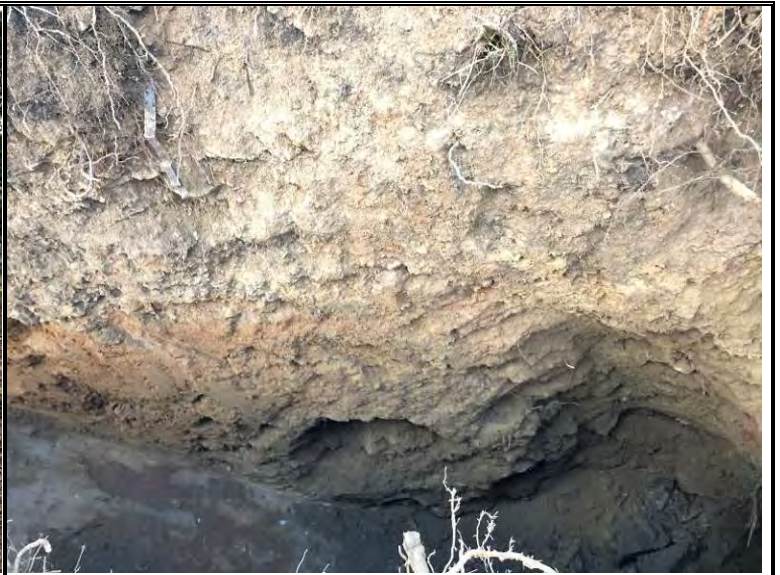
Exposed subsurface soil profile within test-pit TP-11
