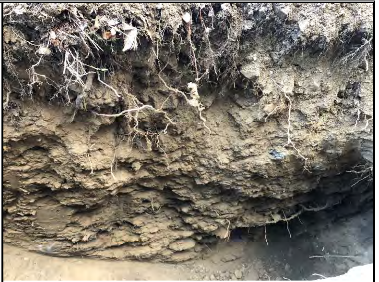
Exposed subsurface soil profile within test-pit TP-4
